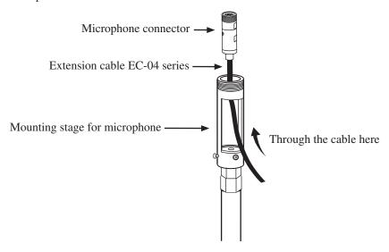
3. Connect the extension cable EC-04 series to the preamplifier.
