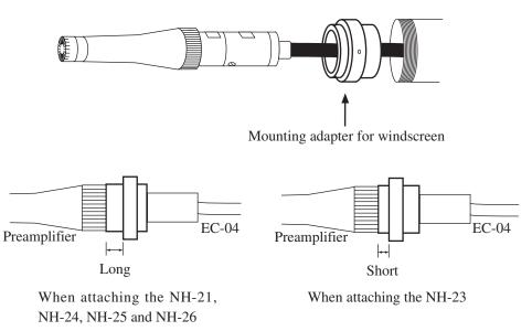
5. Insert the preamplifier into the mounting stage for microphone from the top.
