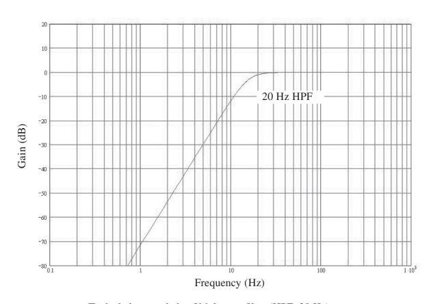
Typical characteristic of high-pass filter (HPF: 20 Hz)
