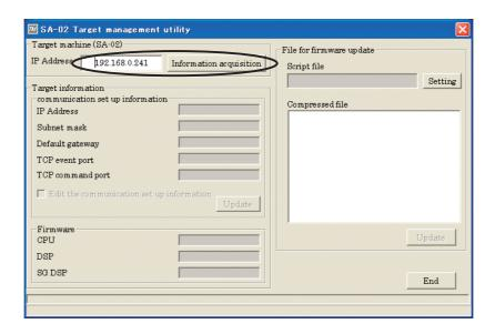
When the connection to the SA-02M/SA-02A4 has been established successfully, the following screen is displayed.
