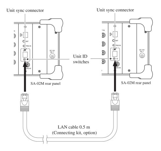
After connecting the LAN cable, set the Unit ID switches. On the unit using channels for 1 to 16, set the Unit ID switch to "1", and set the switch to "2" on the unit using channels for 17 to 32.
