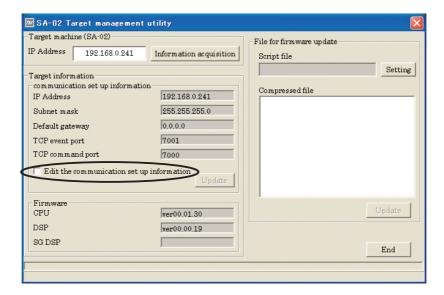
The [Target information] - [communication set up information] field has the following items. Some items can be modified when the [Edit the communication set up information] check box has been selected. Enter the changed value in the respective field and click [Up date].
