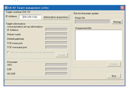
The [Target machine (SA-02)] - [IP Address] field shows the default value: "192.168.0.241"
