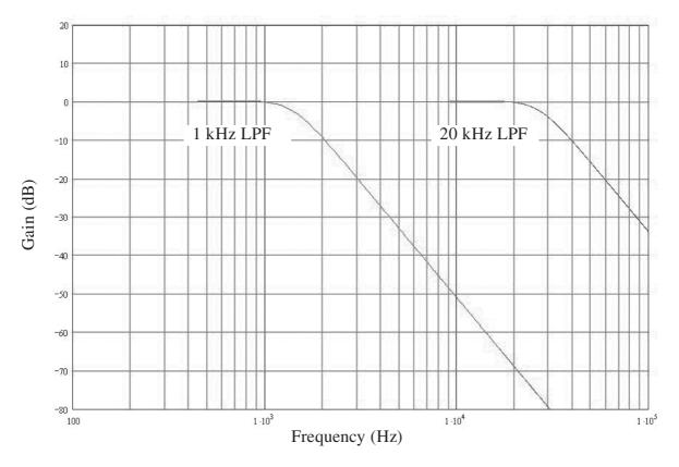
Typical characteristic of low-pass filter (LPF: 1 kHz, 20 kHz)
