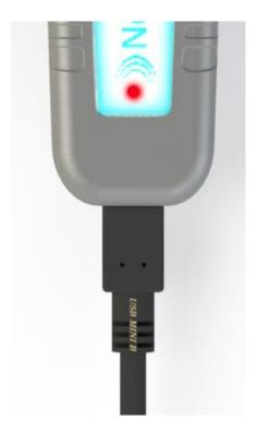
The actual time to fully charge a NoisePen will depend on the current capability of the USB source, but will typically be less than four hours for a fully discharged NoisePen.
