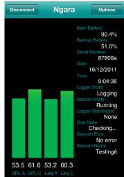
It is possible to configure the amount of data to record before the event occurred (up to 9 minutes), as well as the amount of data to record after the event (up to 9 minutes or continuous)
