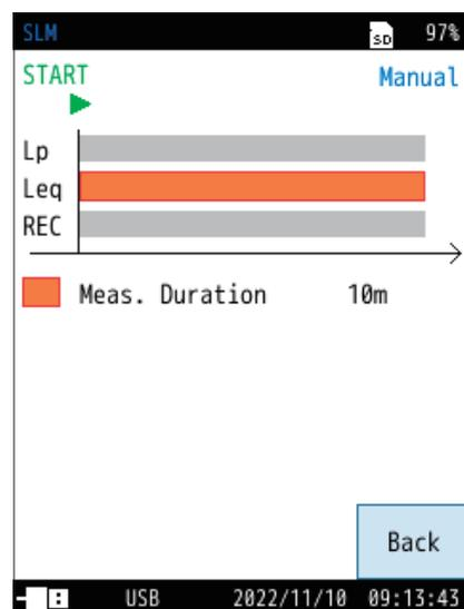
**17** Touch [Back] or press the START/STOP key to return to the measurement screen.
