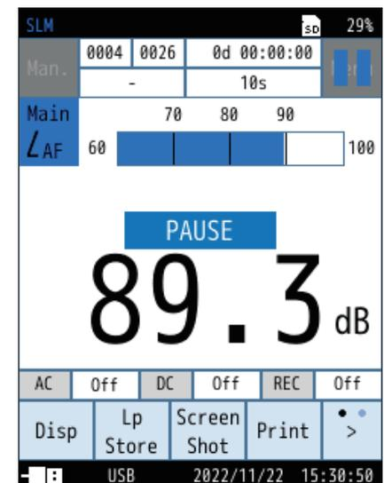
**12** Press the START/STOP key to end the measurement.
