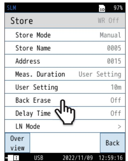
2. Select the back erase time from Off, 1s, 3s, and 5s, and touch [Apply].
