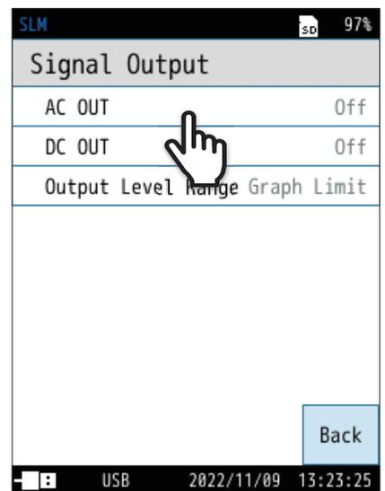
**7** Select the frequency weighting of the AC signal output to the level recorder or data recorder, and touch [Apply].
