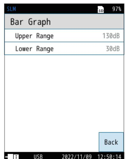
**10** Touch [Back] or press the START/STOP key to return to the measurement screen.
