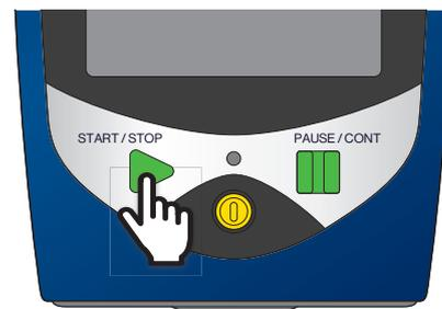
**9** Press the START/STOP key again to end the measurement.
