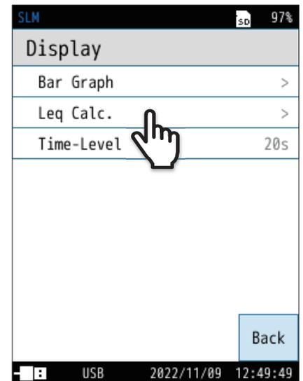
**11** On the [Leq Calc.] screen, set the amount of calculation displayed on the measurement screen to [On].
