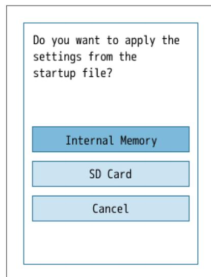
If there is a startup file in the internal memory or on the SD card, a selection screen like the one on the right will appear (the screenshot here is of when the startup file is in the internal memory).
