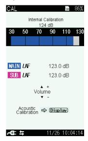
Verify the "Internal Calibration" is displayed in the upper part of the screen.
