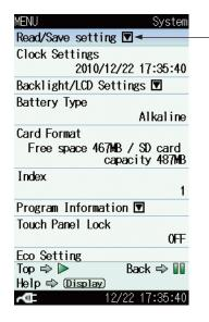
Symbol shows that a next menu level exists. Use  $\triangle/ \bigcirc / \bigcirc / \bigcirc$  keys to select the item and press the MENU/ENT key. The next menu level appears.
