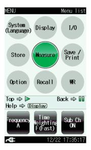
The following settings of Frequency, Time Weighting and Sub Ch can be done with the touch panel. (The current setting is shown when the menu list screen is displayed.) Touch the screen directly with your finger.
