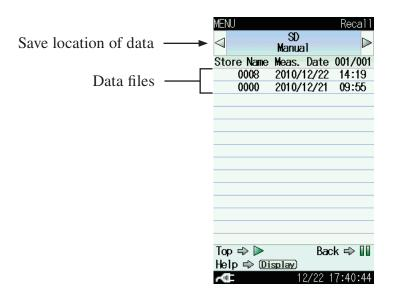
The save location of data can be "Internal Memory Manual", "SD Manual", "SD Auto *L*p" or "SD Auto *L*eq". Without an SD memory card, only "Internal Memory Manual" is available.
