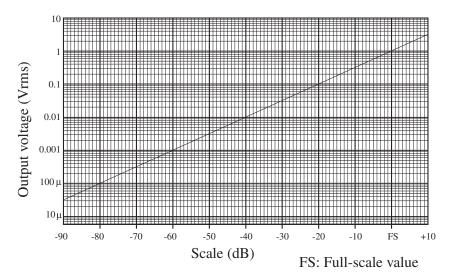
Ideal characteristics of the display value and the output voltage
